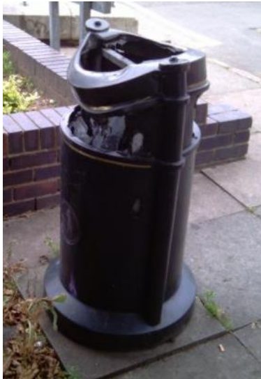
e) Severe damage, causing complete loss of function of the bin
