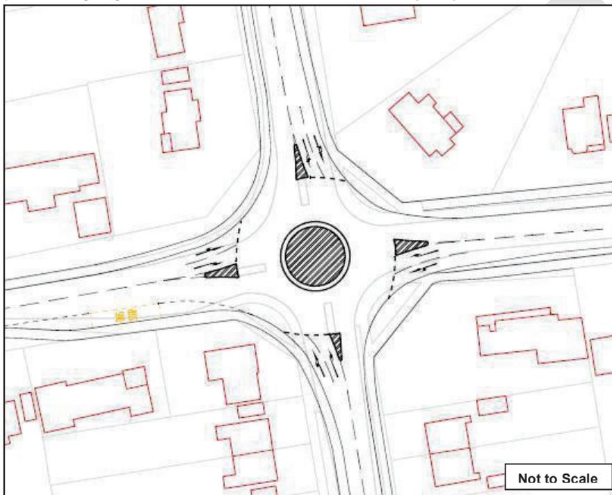
The operational performance of the preliminary design option above has been assessed using ARCADY6. Traffic flows have been input into a model based on the above preliminary design. Table 3.10 summarises the results of the assessments undertaken for the preliminary layout based on the 2031 'Future Base + Development' scenario and compares the results back to the existing layout in the 2031 'Future Base' scenario (i.e. without the additional development traffic).
