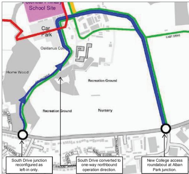
A new access to the College would be created on Hatfield Road at the junction with Alban Park. The existing priority T-junction would be replaced by a roundabout, with a new northern arm serving the College, as shown in Figure 7. This junction would become the main access into the College for staff and students, with only visitors, buses and taxis permitted to use the current access to the west.
