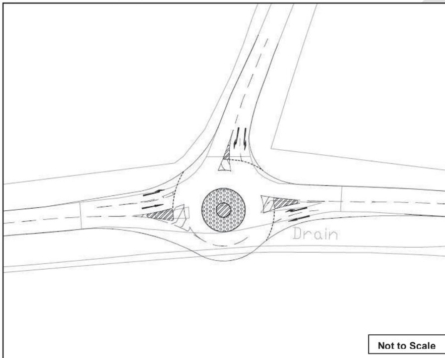
The operational performance of the preliminary design option has been assessed using ARCADY6. Traffic flows have been input into a model based on the above preliminary design. Table 3.7 summarises the results of the assessments undertaken for the preliminary layout based on the 2031 'Future Base + Development' scenario and compares the results back to the existing layout in the 2031 'Future Base' scenario (i.e. without the additional development traffic).
