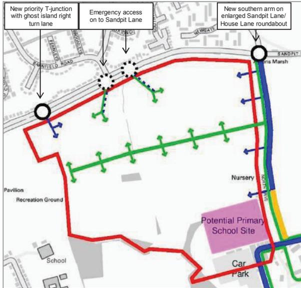
The main access to the initial phase of the development would be located in the north western corner of the site on Sandpit Lane, approximately 200m east of the junction with Damson Way. The junction would be a priority T-junction with a ghost island right turn lane (**Figure 4**).
