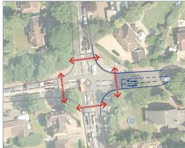
**Figure 18: Sandpit Lane/Marshalswick Lane Junction (Indicative Layout – Compact Roundabout Option)**
