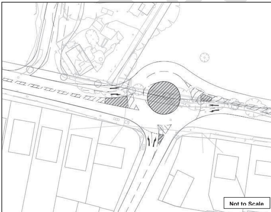
The operational performance of the preliminary design option has been assessed using ARCADY6. Traffic flows have been input into a model based on the above preliminary design. Table 3.11 summarises the results of the assessments undertaken for the preliminary layout based on the 2031 'Future Base + Development' scenario and compares the results back to the existing layout in the 2031 'Future Base' scenario (i.e. without the additional development traffic).
