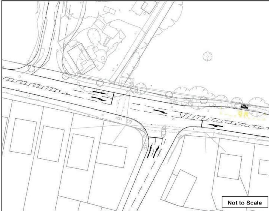
The operational performance of the signalised junction option has been assessed using LINSIG V3 software. Traffic flows have been input into a model based on the above preliminary design. Table 3.12 summarises the results of the assessments undertaken for the preliminary layout based on the 2031 'Future Base + Development' scenario and compares the results back to the existing layout in the 2031 'Future Base' scenario (i.e. without the additional development traffic).
