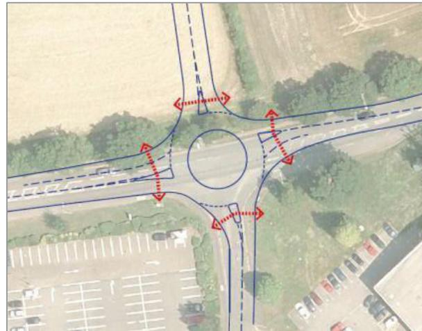
**Figure 8: Hatfield Road/Colney Heath Lane Junction (Indicative Layout – Roundabout Option)**
