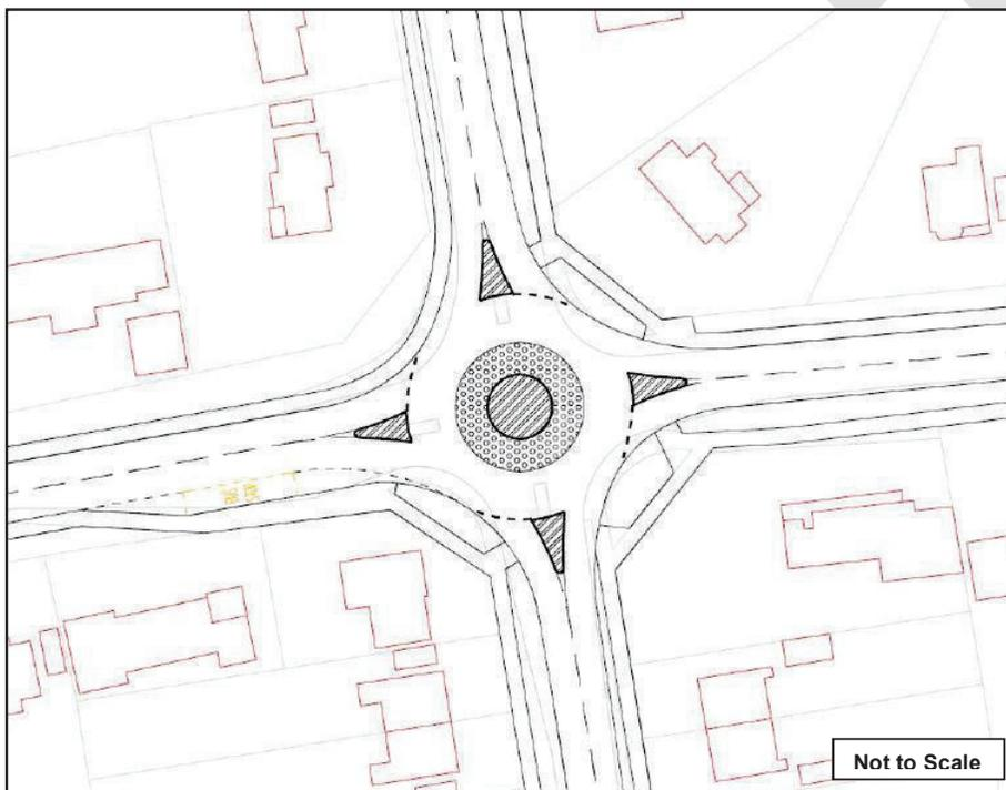
The operational performance of the preliminary design option above has been assessed using ARCADY6, which is the industry standard software for assessing priority roundabouts. Table 3.9 summarises the results of the assessments undertaken for the preliminary layout based on the 2031 'Future Base + Development' scenario and compares the results back to the existing layout in the 2031 'Future Base' scenario (i.e. without the additional development traffic).
