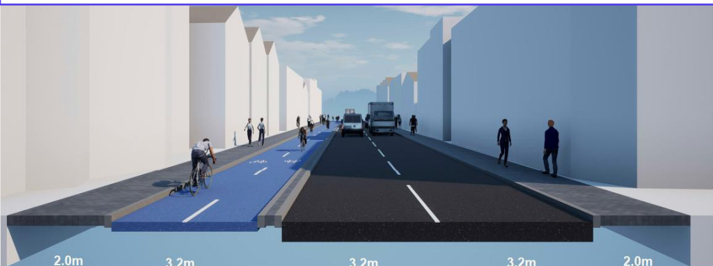
Example Ideal Cross-Section with Two-Way Cycle Track (Kerb Protected) Source: ATE cross-section check. Visualisations prepared by Mott MacDonald Group
