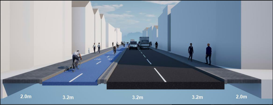
Example Ideal Cross-Section with Two-Way Cycle Track (Kerb Protected) Source: ATE cross-section check. Visualisations prepared by Mott MacDonald Group
