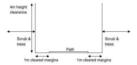
Diagram: Minimum standard of maintenance along the route.
