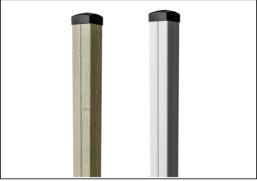
The main tower posts are available in two types of material: Pine wood posts pressure impregnated class AB with Tanalith E3475 according to EN335. Aluminum post t=2mm with anodized surface treatment. Base material EN AW-6060 T66.
