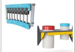
The Xylophone music panel consist of HDPE material in 19mm EcoCore ™. The pipes are made of die cast aluminum specifically alloyed for outdoor environments. The percussion panel consist of 2 Conga Drums with PP tubes and top in colored ABS.
