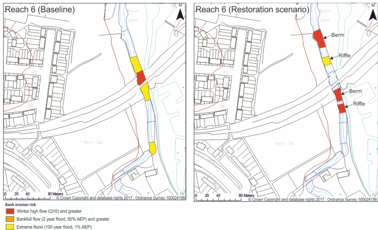
Figure 53. Sedimentation risk at Reach 6 under baseline and proposed restoration scenarios. Note: Model results also indicated low shear stress values under summer low flow conditions, however this is not likely to result in such widespread sedimentation given the low volume of flow and reduced sediment volumes being transported within the low flow channel. As such, only sedimentation risks associated with a winter high flow or bankfull flow have been identified.
