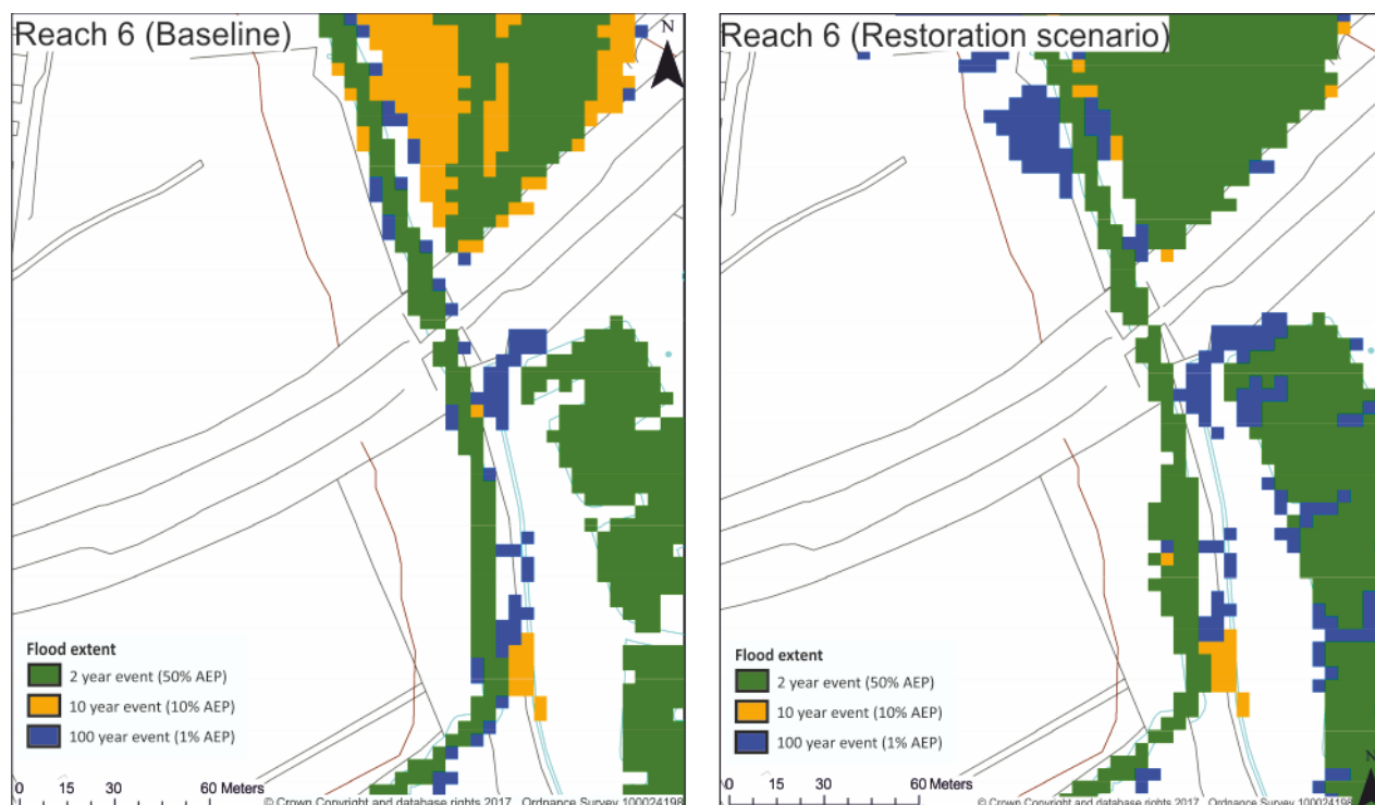
Figure 50. Flood modelling results at Reach 6 under baseline and proposed restoration scenarios (increased areas of yellow indicate increased flood extent at the 2 year RP flow and increase in blue area is related to increased flood extent at the 100 year RP flow)
