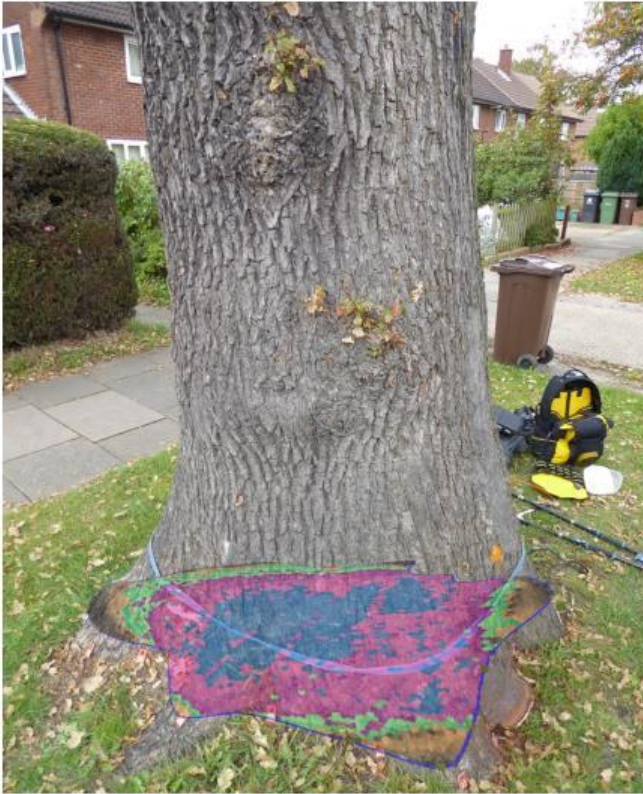
T2784 oak tree Cell Barnes Lane PiCUS: sonic tomogram (right) superimposed in approximate position over the stem (left).
