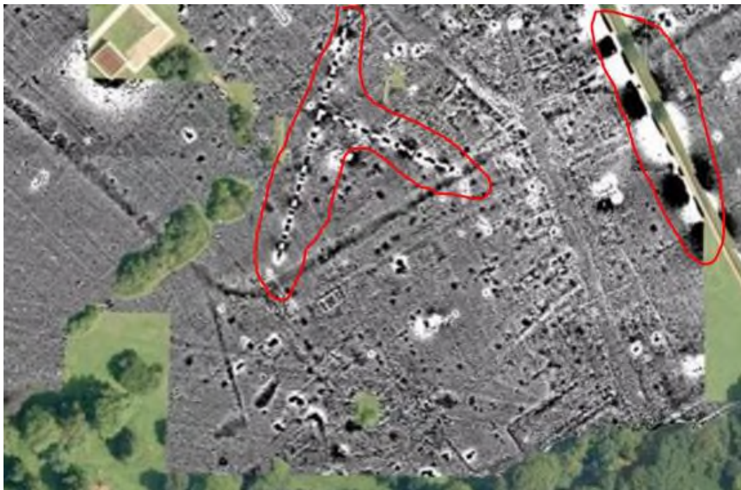
The survey has also helped us to identify the positions and routes of water mains, seen in the middle of this image. The 8" gas main can also be clearly seen to the right, running under the the footpath.
