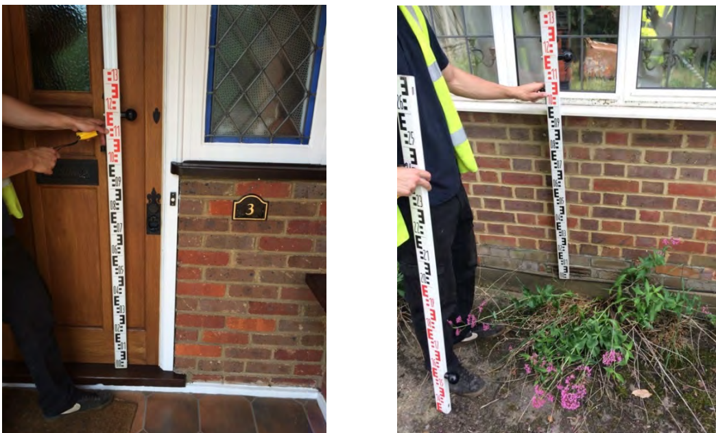
Photograph 14: Surveying of property threshold levels for use in flood modelling
