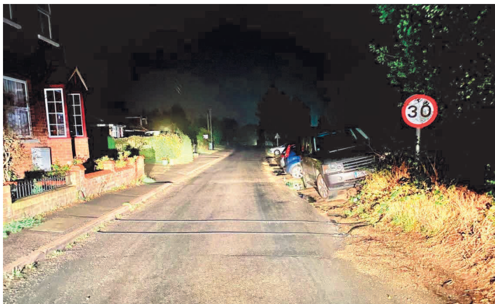
Figure 19 View of ATC Installed along Chiswell Green Lane
