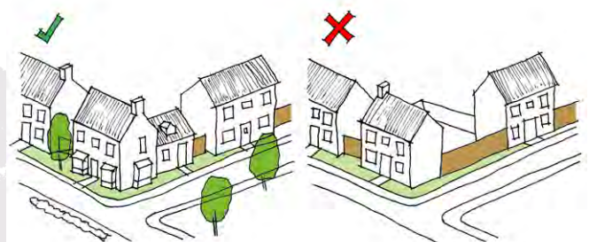
Figure 27: Active frontage onto streets and spaces
