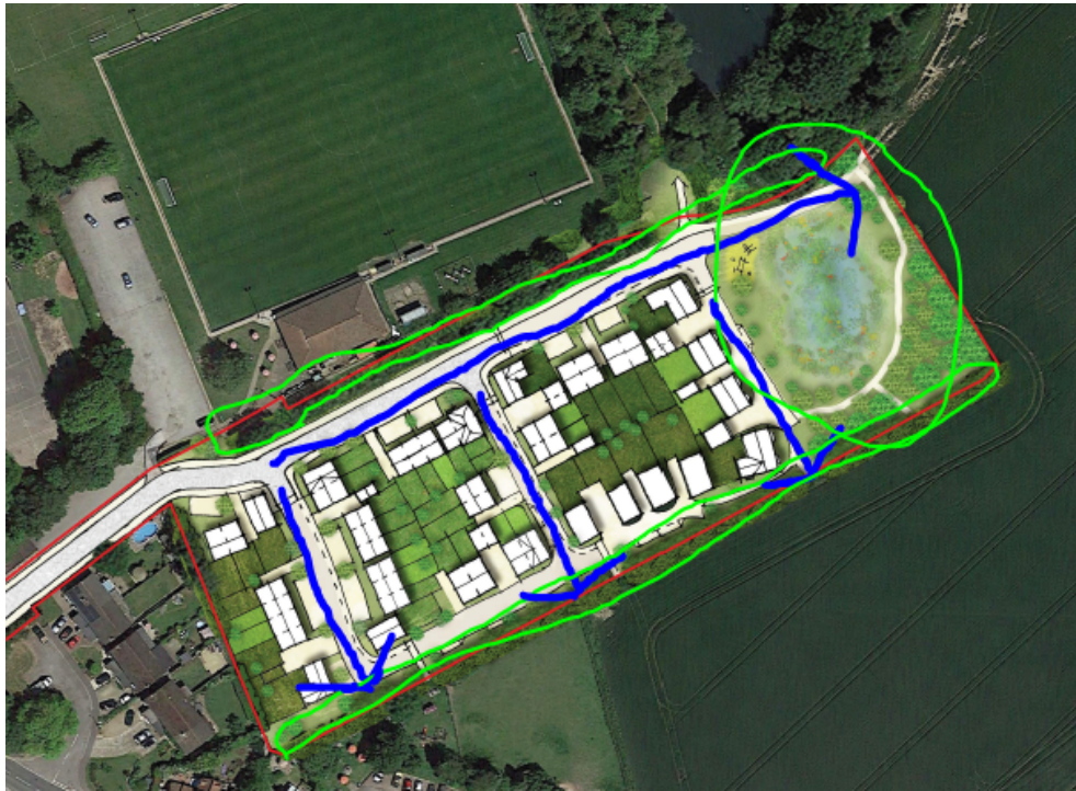
Figure 5.2: Open spaces and open view lines which could be integrated into the development to maintain a degree of physical and visual openness and create an open character
