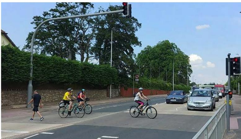
**20.2** A Toucan Crossing should only be used where options which do not involve sharing space between pedestrians and cyclists (such as a parallel or signalised parallel crossing) have been thoroughly examined and found to be undeliverable in a specific location.
