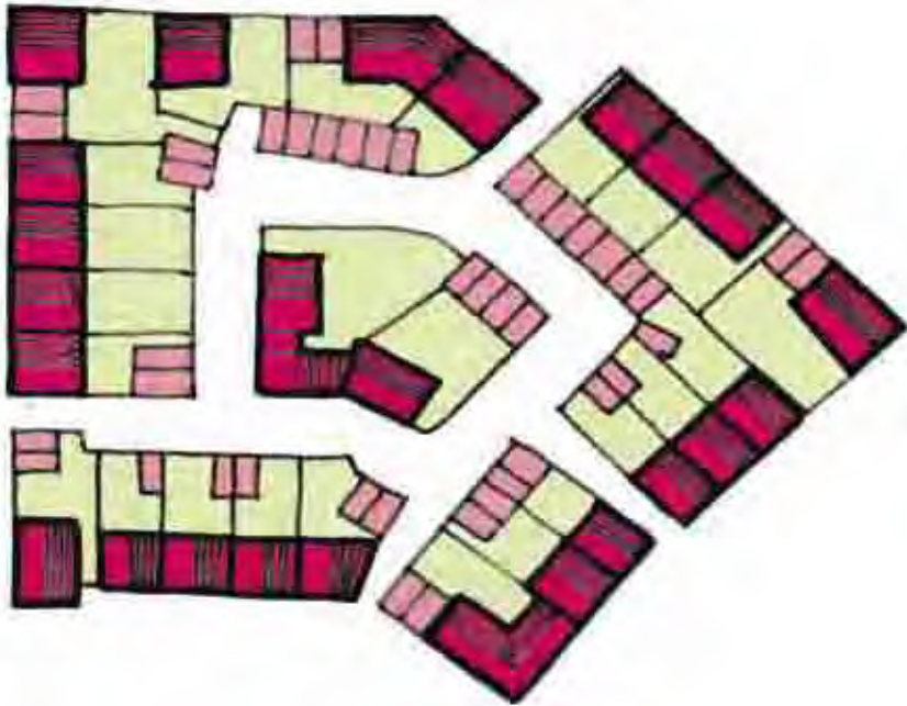
Figure 8.12 This arrangement of buildings creates well-overlooked parking spaces (shown in pink) – through routes increase natural surveillance from passing pedestrians (source: Better Places to Live ).
