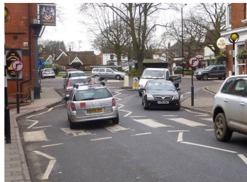
Plate 3 - Poor alignment on southern side(left) leaving dead area of carriageway
