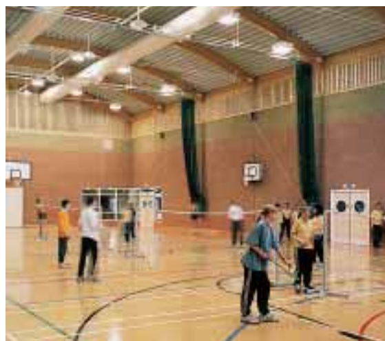
Sports hall structure, lights and division netting must be aligned between badminton courts.
